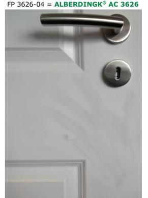
\*16h Alberdingk-fatty acid test which simulates the resistance of the film to human hand fat or hand lotions.
